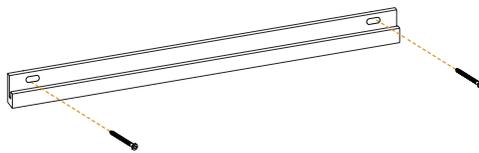
Screw the lower list onto the wall.
