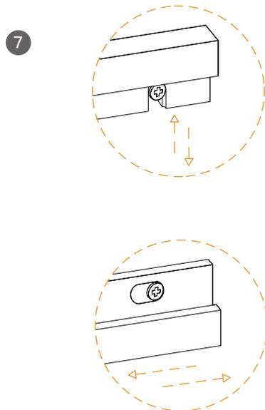
If the lists are not completely aligned, simply adjust the positions of them by sliding the elongated holes along the screws.
