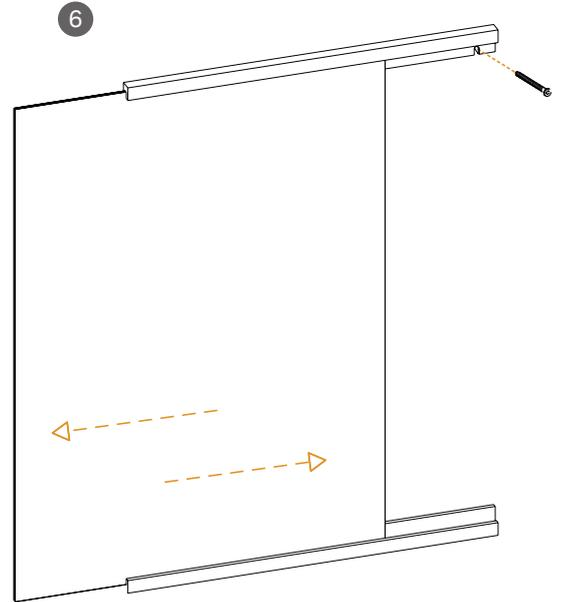
Place both the mirror and the upper list loosely on the bottom list, remember to hold it in place to prevent it from falling. Slide the mirror to both sides and screw the upper list onto the wall. Lastly, slide the mirror glass into place.
