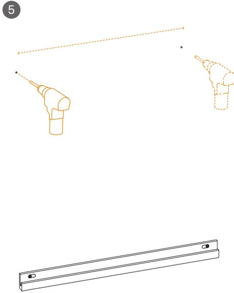
Drill the two holes and insert adequate wall plugs suited for you wall type.
