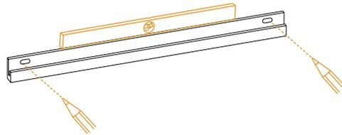
Hold the lower list - the list with horizontal holes - against the wall, make sure it is leveled. Use the two holes to mark where to drill.
