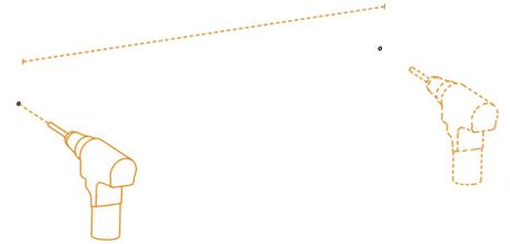
Drill the two holes and insert adequate wall plugs suited for you wall type.
