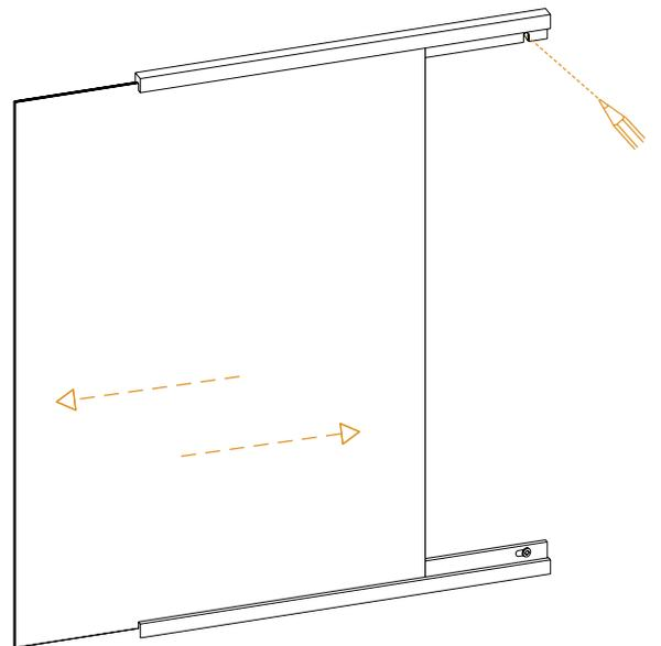
Place both the mirror and the upper list - the list with vertical holes - loosely on the bottom list, remember to hold it in place to prevent it from falling. Slide the mirror to both sides and mark where to drill.
