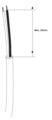
Trim the cable to the desired length, leaving 35mm of basic single insulation exposed for wiring.
